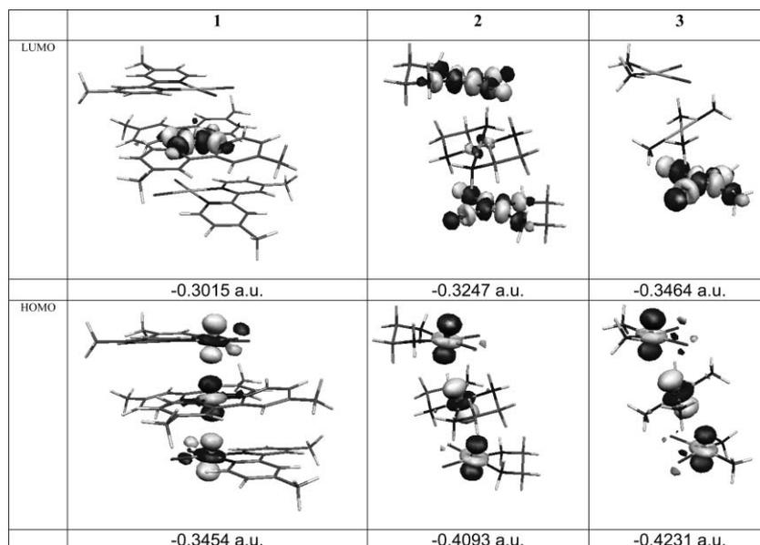
**Fig. 4** HOMO and LUMO molecular frontier orbitals for complexes **1**, **2**, and **3**. Isosurface values are  $-0.05$  a.u. and  $0.05$  a.u.
