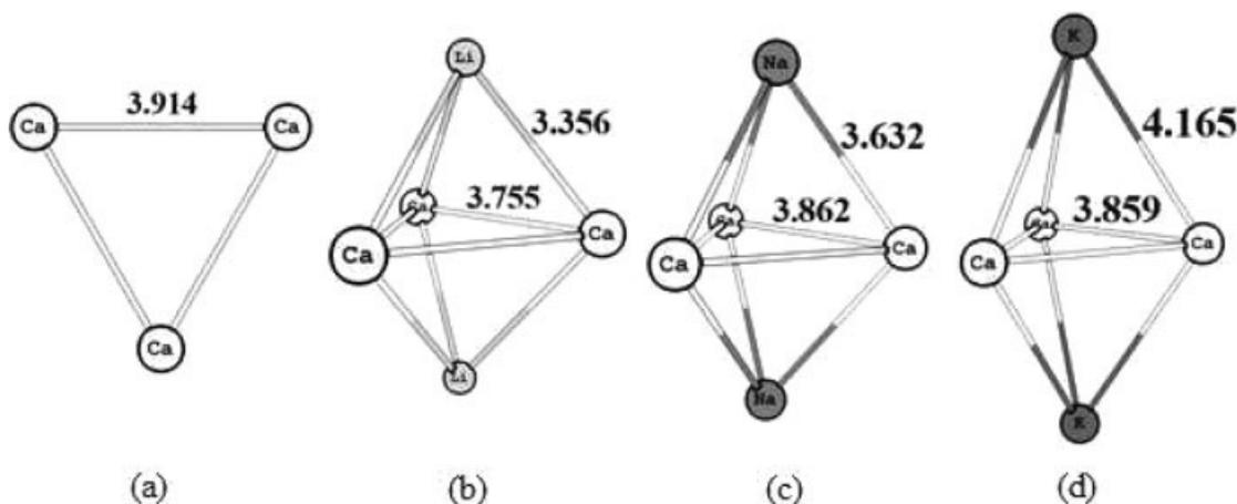
**Figure 6.** B3LYP/6-311+G(d) optimized structures of calcium species for (a) trigonal planar  $\text{cyclo-}[\text{Ca}_3]^{2-}$  ( $D_{3h}, {}^1A_1'$ ), (b) bipyramidal  $\text{Li}_2\text{Ca}_3$  ( $D_{3h}, {}^1A_1'$ ), (c) bipyramidal  $\text{Na}_2\text{Ca}_3$  ( $D_{3h}, {}^1A_1'$ ) and (d) bipyramidal  $\text{K}_2\text{Ca}_3$  ( $D_{3h}, {}^1A_1'$ ). Bond lengths are given in Å.
