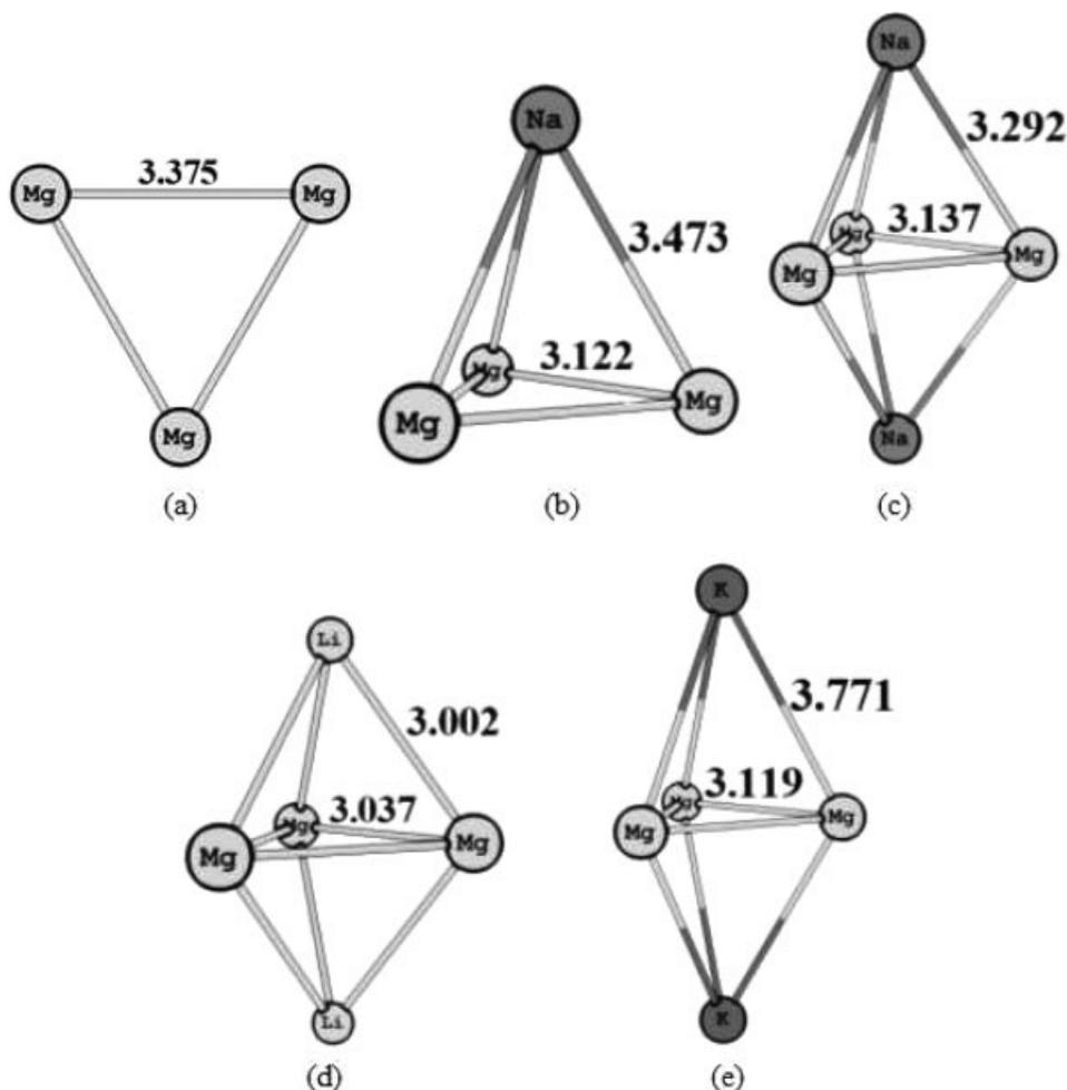
**Figure 1.** B3LYP/6-311+G(d) optimized structures for (a) trigonal planar  $\text{cyclo-}[\text{Mg}_3]^{2-}$  ( $D_{3h}$ ,  $^1A_1'$ ), (b) trigonal pyramidal  $\text{NaMg}_3^-$  ( $C_{3v}$ ,  $^1A_1$ ), (c) bipyramidal  $\text{Na}_2\text{Mg}_3$  ( $D_{3h}$ ,  $^1A_1'$ ), (d) bipyramidal  $\text{Li}_2\text{Mg}_3$  ( $D_{3h}$ ,  $^1A_1'$ ), and (e) bipyramidal  $\text{K}_2\text{Mg}_3$  ( $D_{3h}$ ,  $^1A_1'$ ). Bond lengths are given in Å.
