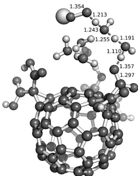
Figure 5. BP86/TZP-optimized geometry including DMSO as solvent of the transition state **TS1** that involves proton transfer from a  $C_3$  carboxyl group towards the superoxide radical through two bridging water molecules; relevant distances [Å] are indicated by dotted lines.
