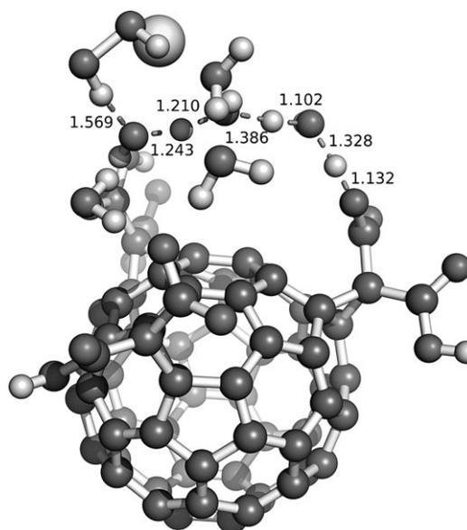
Figure 7. BP86/TZP-optimized geometry including DMSO as solvent of the transition state **TS3** that involves subsequent proton transfers from one protonated carboxyl group of  $C_3$  to the deprotonated water molecule that in **TS2** transferred one of its hydrogen atoms to the hydroperoxide anion to form hydrogen peroxide; relevant distances [Å] are indicated by dotted lines.
